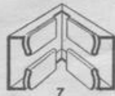
7 FOUNDATION CORNER BRICK
